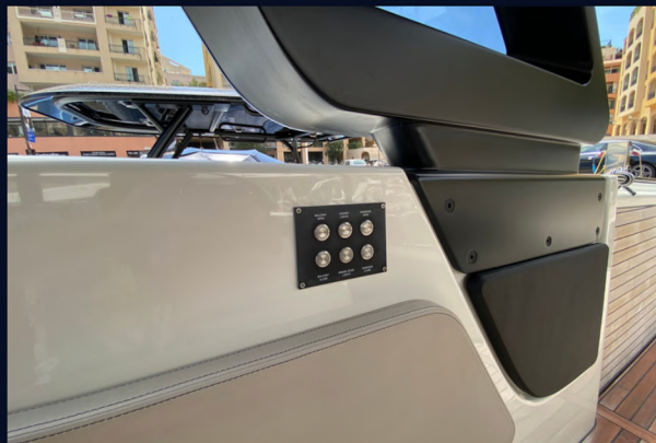
[Electric Roof Controls]
