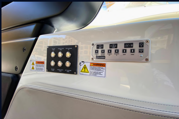
[Gangway & Rear Hatch Controls]
