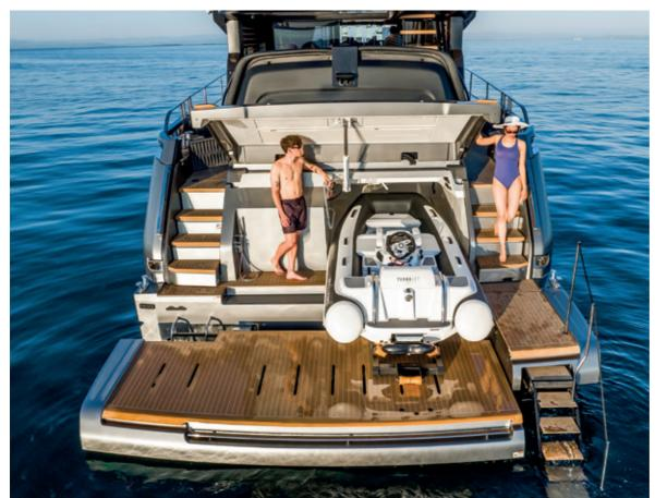
LA PASSERELLA **IDRAULICA A** SCOMPARSA REALIZZATA DA BESENZONI. **UNA VOLTA** ESTRATTA, FUNGE DA SCALETTA PER SBARCARE IN BANCHINA. **OPPURE COME SCALETTA** BAGNO. ONCE EXTENDED, THE FOLDABLE **HYDRAULIC GANGWAY** BY BESENZONI **BECOMES A** LADDER FOR **DISEMBARKING** ON THE QUAY OR A BATHING LADDER.
